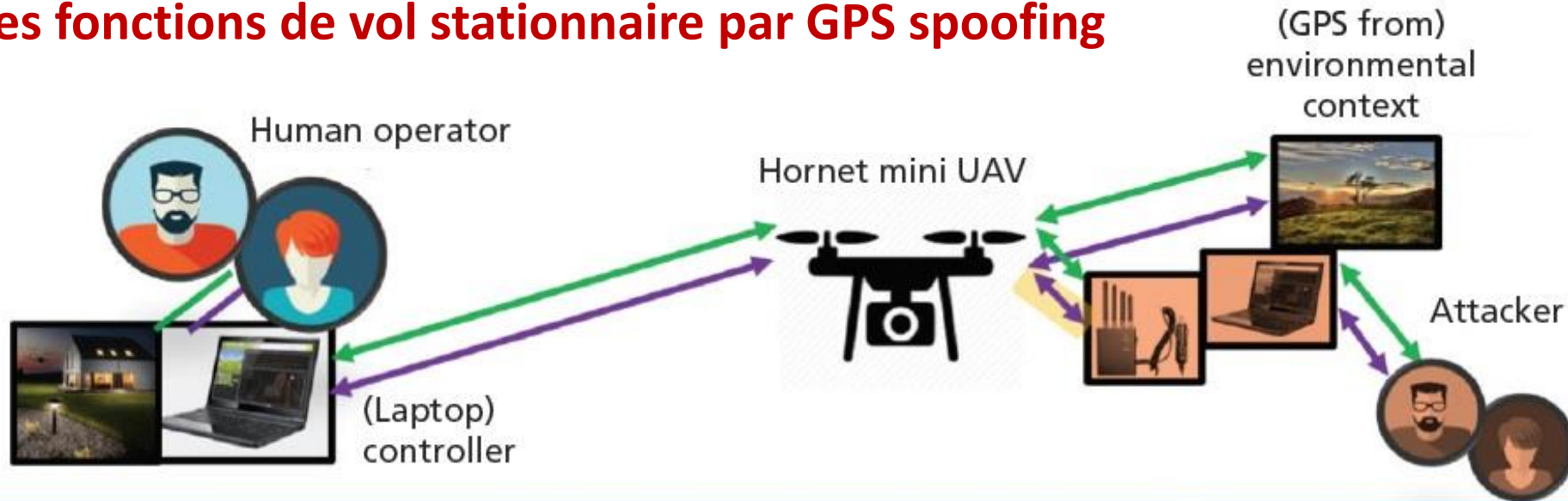
Spoofing – UAS as target – false GPS data injection over standard GPS signal (Sensor)
